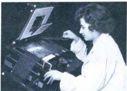
Photographic training is given to women members of the Royal Air Force, one of whom is seen here operating a machine for contact printing 5-in. wide perforated film, used in many air-to-ground cameras.
