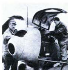
The Cameras Are Fitted Photographs are taken vertically and at an angle to build up a complete mosaic of the target area.
